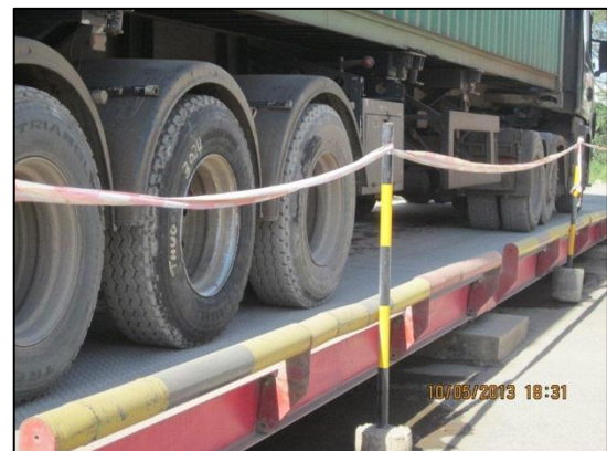
A Truck entering the ramp of the Weighing Platform (left Photograph). Second Photograph on the right shows the Pit-less platform and the three groups of axles on three sections of the platform
