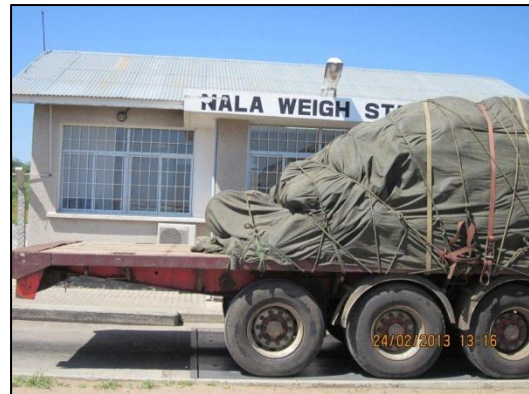
Truck axles – Front single axle in the left photograph and tridem axle in the right photograph standing on the single platform Weigh-Bridge installed in a pit
