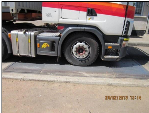
Truck axles – Front single axle in the left photograph and tridem axle in the right photograph standing on the single platform Weigh-Bridge installed in a pit
