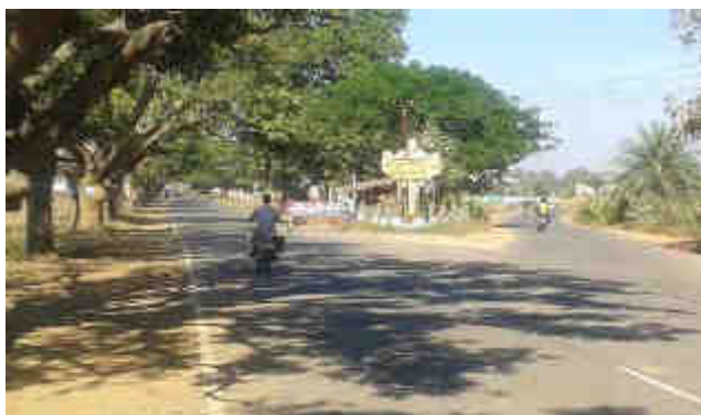
Km 316+900, intersection of NH-49 with Kuchinda town road (south of Kuchinda) – non-standard island with buildings and trees obstructing visibility
