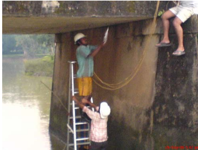
Rebound Hammer testing in Deck slab for bridge at Ch.6/050
