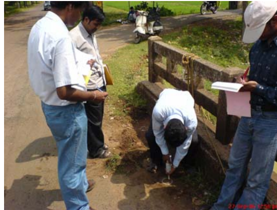
Rebound Hammer testing in deck slab for bridge at Ch. 19/300
