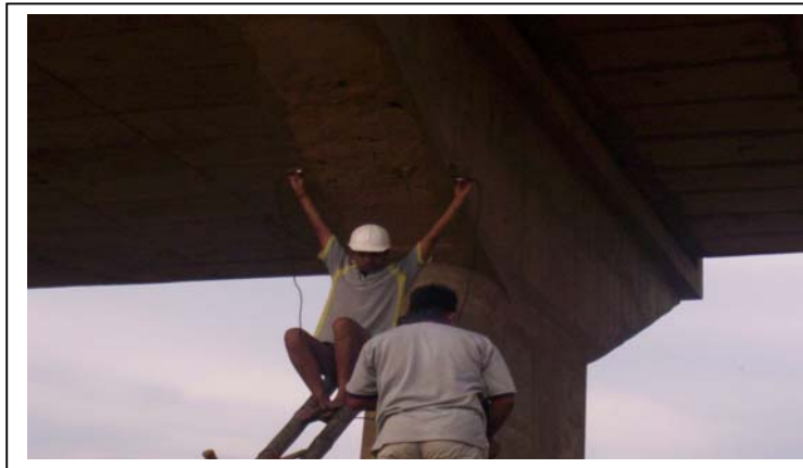
Pulse velocity Test in Pier cap for bridge at CH. 27/850
