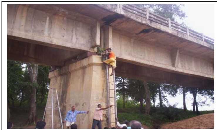
Rebound Hammer testing in Deck slab for bridge at Ch. 59/100
