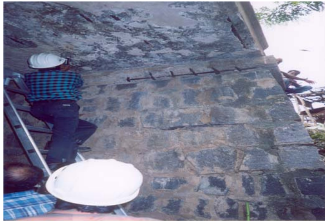
Pulse velocity Test in deck slab for bridge at Ch. 11/270
