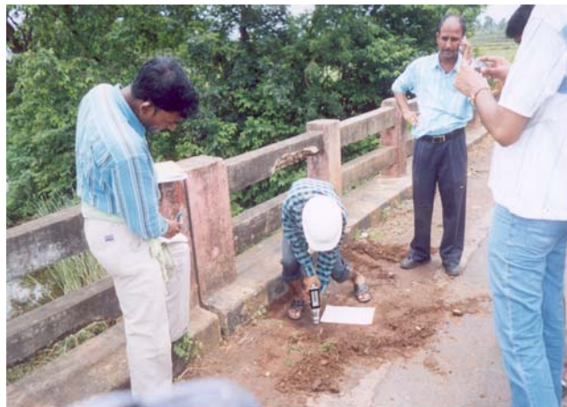
Rebound Hammer testing for bridge at Ch. 17/900
