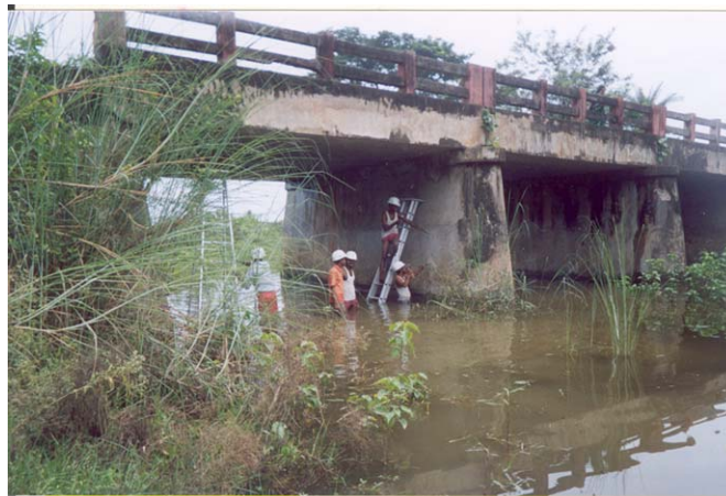
Pulse velocity Test for bridge at CH. 17/900
