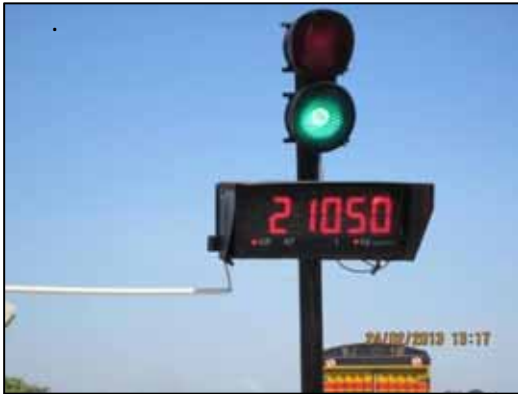
Monitor on the left indicating the combined load of the tridem axle and the green light indicating the load being within the permissible limits as being also seen inside the weigh-bridge control room
