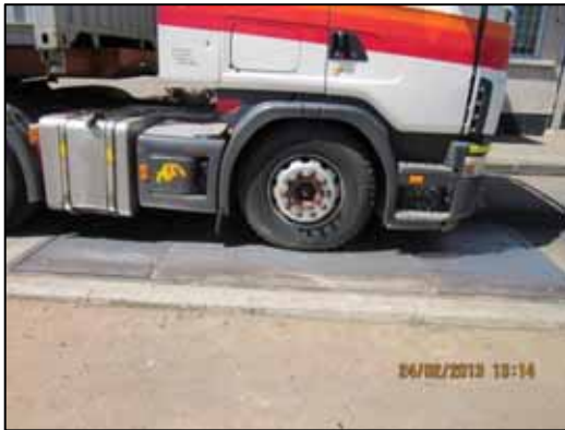
Truck axles – Front single axle in the left photograph and tridem axle in the right photograph standing on the single platform Weigh-Bridge installed in a pit
