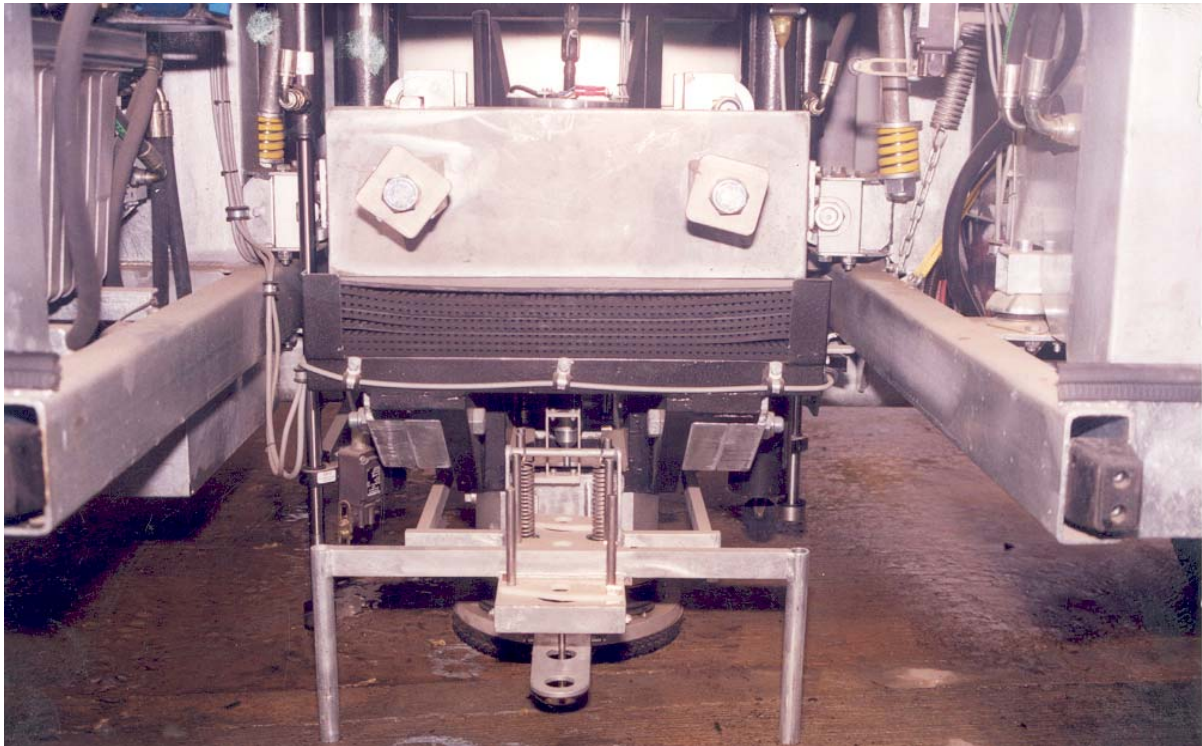
Sensor Bar in Contact with Pavement Surface
