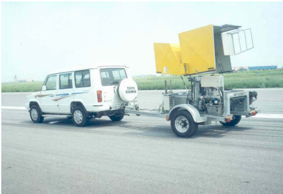
Falling Weight Deflectometer (FWD) in use
