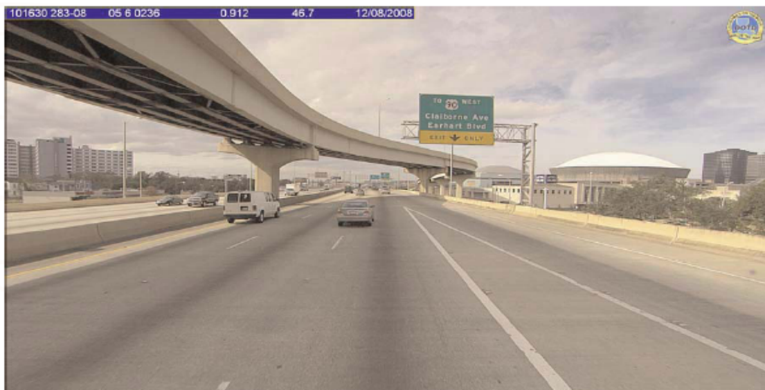
Pictured here: 1920 x 1080 pixel resolution (HDTV) Right-of-Way video image, with 90 degree horizontal field of view
