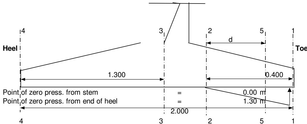
**DESIGN OF TOE SLAB****Reinforcement calculation**
