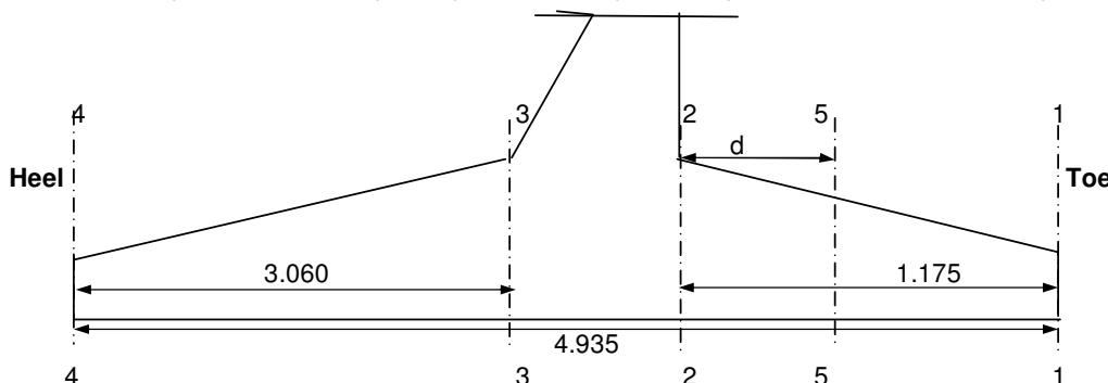
**DESIGN OF TOE SLAB****Reinforcement calculation**
