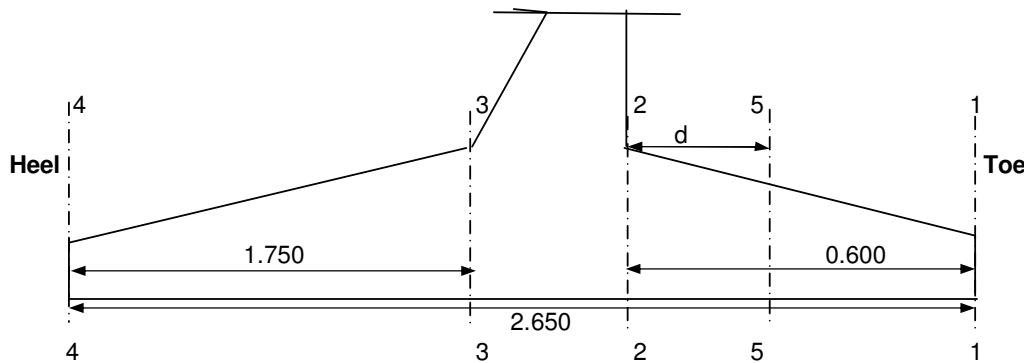
**DESIGN OF TOE SLAB****Reinforcement calculation**
