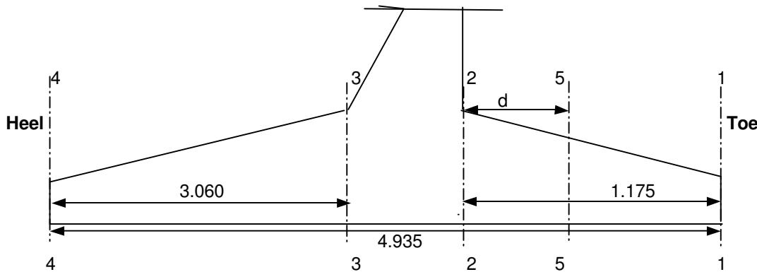
**DESIGN OF TOE SLAB****Reinforcement calculation**
