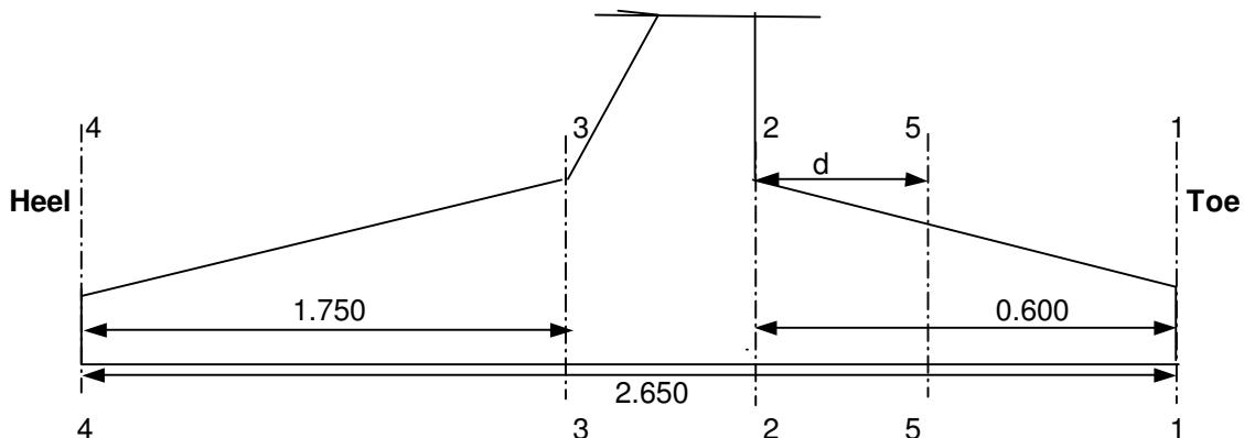
**DESIGN OF TOE SLAB****Reinforcement calculation**
