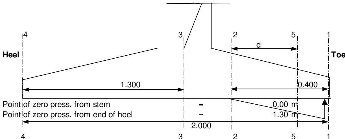
**DESIGN OF TOE SLAB****Reinforcement calculation**
