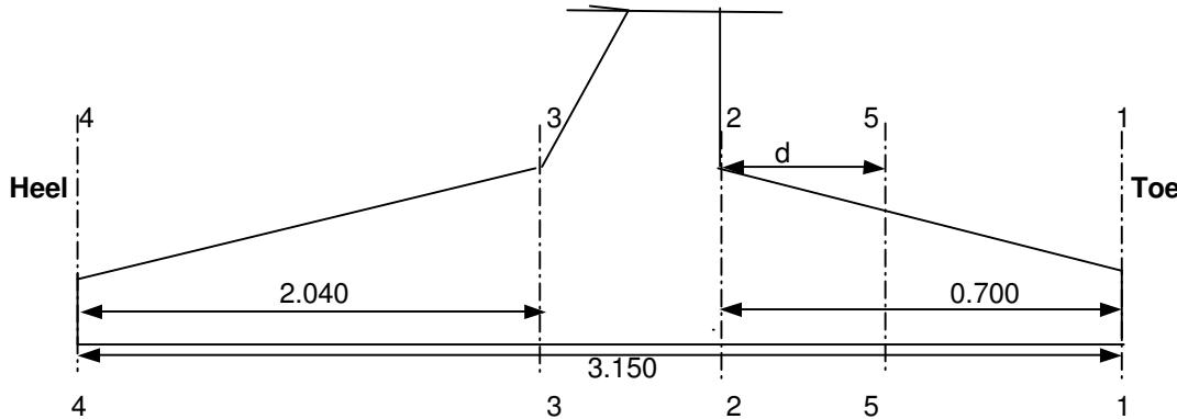
**DESIGN OF TOE SLAB****Reinforcement calculation**
