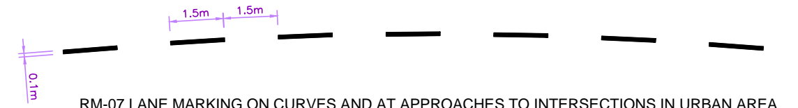
RM-07 LANE MARKING ON CURVES AND AT APPROACHES TO INTERSECTIONS IN URBAN AREA
