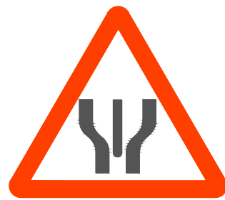
START OF DUAL CARRIAGEWAY
